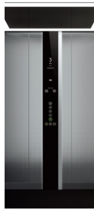
Alto full height Surface mounted full-height COP, black glass faceplate with st. steel edge, 7" TFT display. Two widths for up to 18 or 24 buttons. Optional LED backlight.
